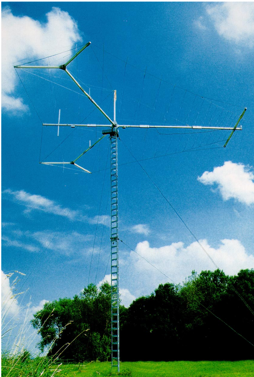
Antenna System AK451: Rotatable Log-periodic Antenna HL451 (5 to 30 MHz), mounted on a 15-m mast; comparison with previous antennas (diagram on the right) confirms massive reduction of antenna size
